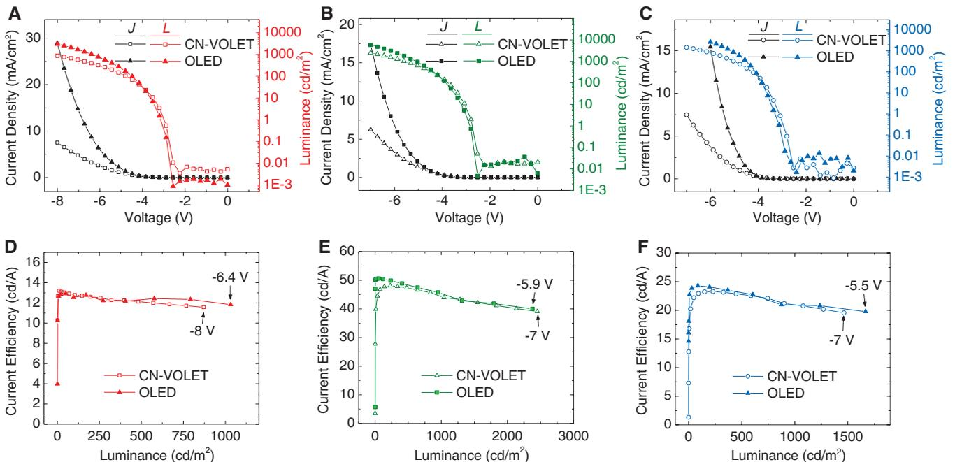
**Fig. 3.** Comparison of the CN-VOLETs to control OLEDs.  $J$ - $L$ - $V$  comparison for the (A) red, (B) green, and (C) blue CN-VOLETs in the on state (i.e.,  $V_G = -3$  V) to their respective OLEDs. Applied voltage is on the drain of the CN-VOLET (source grounded)
